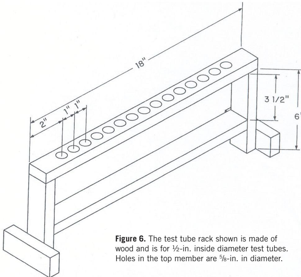
**Figure 6.** The test tube rack shown is made of wood and is for  $\frac{1}{2}$ -in. inside diameter test tubes. Holes in the top member are  $\frac{5}{8}$ -in. in diameter.
