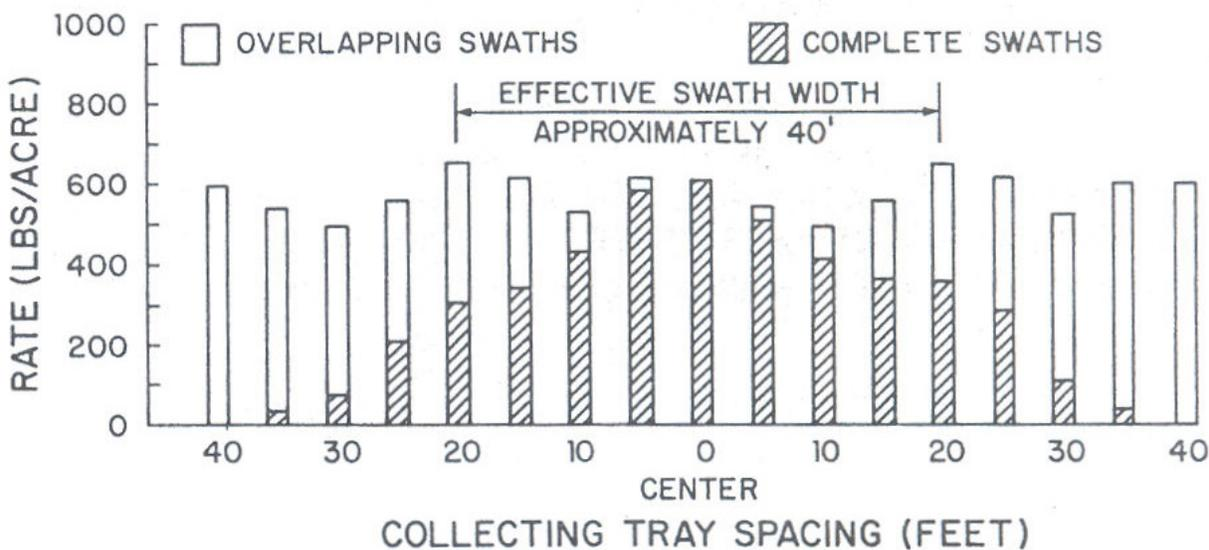
**Figure 2.** The spread pattern is determined by collecting the material in trays/pans and pouring it into test tubes. Material overlap, as shown, results when swath spacing equals the effective swath width. This is a typical pattern one might expect from a dual spinner-disc fertilizer spreader. This does not depict an ideal pattern.
