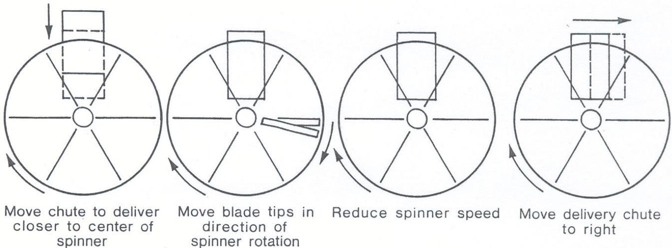
**Figure 5.** Four adjustments to correct heavy right distribution patterns from a single spinner-disc fertilizer applicator. These four corrections allow material to ride the spinner further and deposit toward the left side. Corrections for heavy left patterns are opposite to those shown for heavy right patterns.
