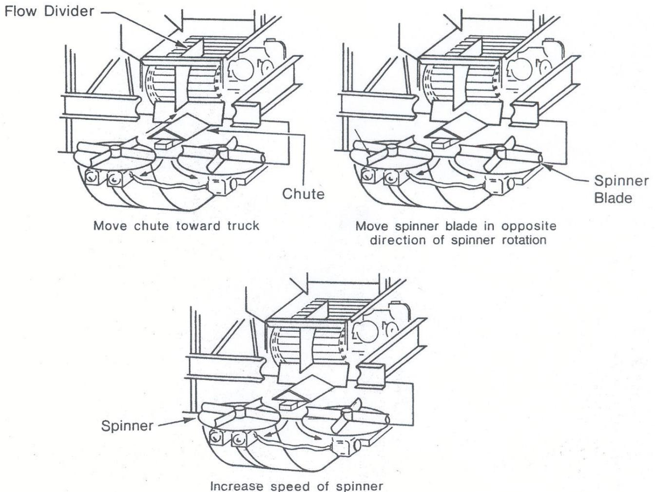
**Figure 4.** Dual spinner-disc fertilizer applicator showing adjustments for corrections of an M distribution pattern, characterized by low delivery in the center and high delivery on the edges of the swath.
